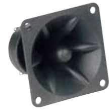
GT2-1046 Frequency Response: 4.5-20KHz Sensitivity: 102dB(1w/1m) Power RMS/MAX: 75/150w Impedance: 4 Ohm Size: \phi 85 \times 85 mm
