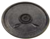
GT2-1031 (XH50-4) 2" Telephone speaker 16 ohm 0.4W magnet NdFeB: \phi 12 \times 1.5 mm Dimension: \phi 50 \times 9 mm
