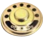
GT2-1031 (XH50-4) 2" Telephone speaker 16 ohm 0.4W magnet NdFeB: \phi 12 \times 1.5 mm Dimension: \phi 50 \times 9 mm
