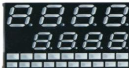
The LED display and LED indicators was built as one panel ,most of controller with their LED display and LED indicator installed separately, the chance of the malfunction is high. This controller with all the display and indicator units built together on board, makes it easier to install and easy to test with higher reliability.
