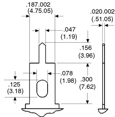
Printed Circuit Terminal For direct relay to PCB mounting. Model 157-9
