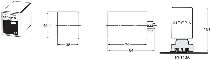
When mounting a Display Unit to a PF113A Surface-mounting Socket, secure the PF113A with the groove facing toward the bottom and then connect the 61F-GP-N the PFC-N8 accessory.
