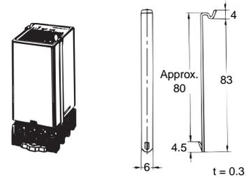
**Note:** PFC-N8 Mounting Bracket (provided with the Level Controller)
