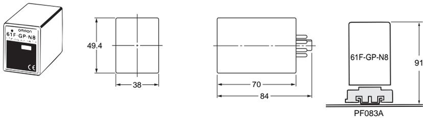
Use a PFC-N8 Mounting Bracket to mount the Level Controller to a PF083A Rail-mounted Socket.
