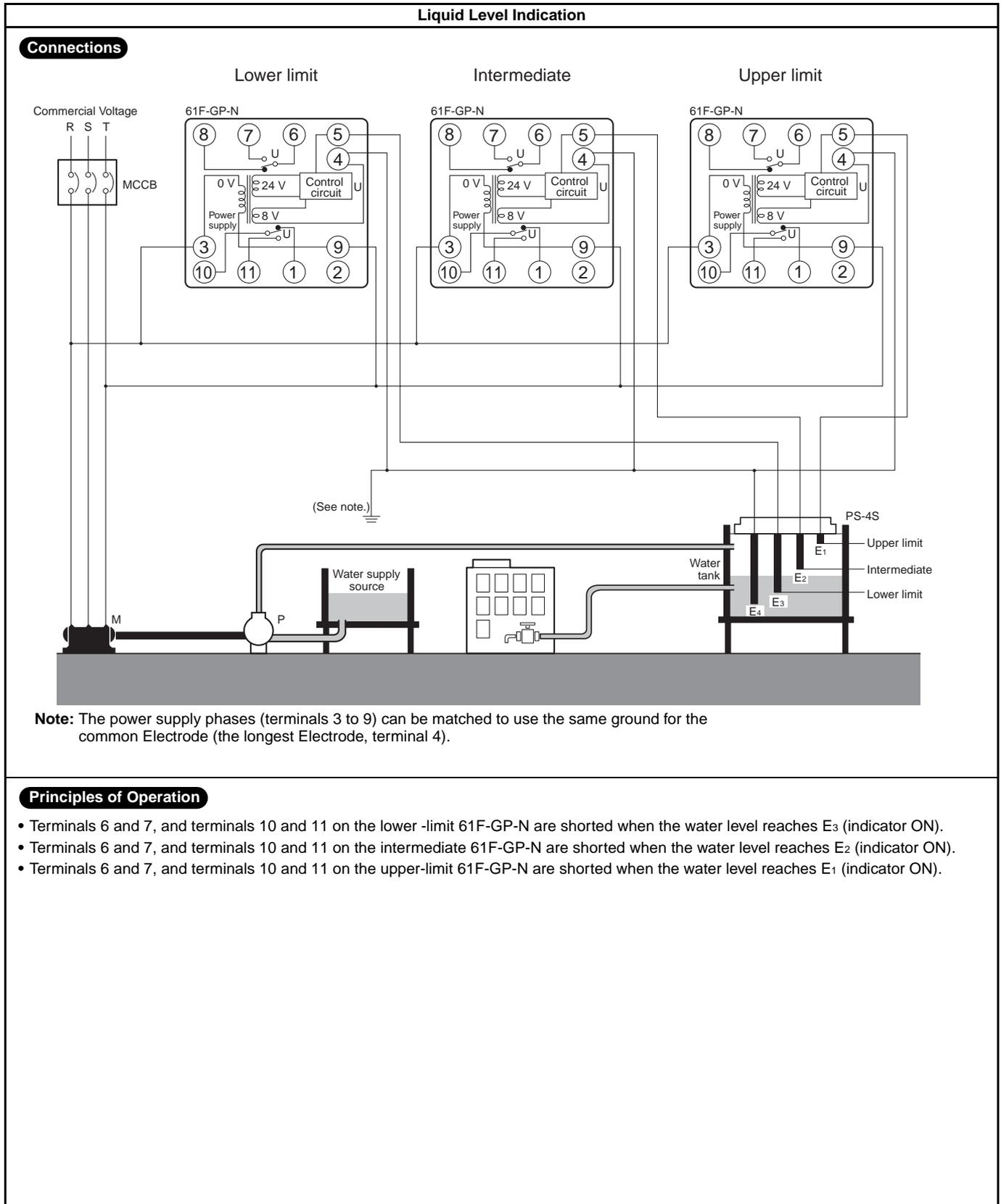
**Replacing 61F-G3N Functions (Automatic Water Supply Control with Abnormal Water Increase and Water Shortage Alarms)**
