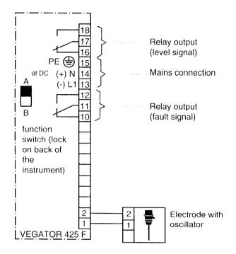
The electrical connections should be made on the mounting assembly in accordance with the diagram located on the back of the instrument.
