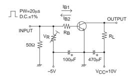
$7I_{B1} = -7I_{B2} = I_{C} = 700 \text{mA}$
