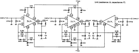
$\begin{array}{ll} \text{Vo:} & \text{V}_{NO} \text{ is measured by connecting a VTVM.} \\ & \text{V}_{N} \text{ is measured by connecting a DC voltmeter.} \\ & t_{D} \text{ is measured by connecting an oscilloscope.} \end{array}$
