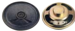
GT2-1032 (XH50-5) 2" Telephone speaker 8 ohm 1W magnet NdFeB: \phi 12 \times 2 mm Dimension: \phi 50 \times 17.5 mm
