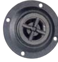
GT2-1045 Frequency Response: 4.5-20KHz Sensitivity: 103dB(1w/1m) Power RMS/MAX: 75/150w Impedance: 4/8 Ohm Size: \phi 80 mm
