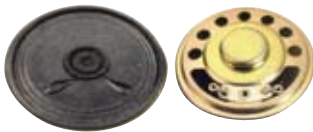
GT2-1031 (XH50-4) 2" Telephone speaker 16 ohm 0.4W magnet NdFeB: \phi 12 \times 1.5 mm Dimension: \phi 50 \times 9 mm
