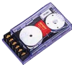
GT2-1070 (SH617) 120W 2WAY W.: 6dB/OCT T.: 12dB/OCT FREQ.: 5.5KHz IMPEDANCE: 4/8 \Omega
