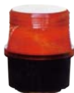
GT2-1131 (XH-80) *6-12VDC 250mA 90Flashes/min *Color:Red,Blue,Yellow
